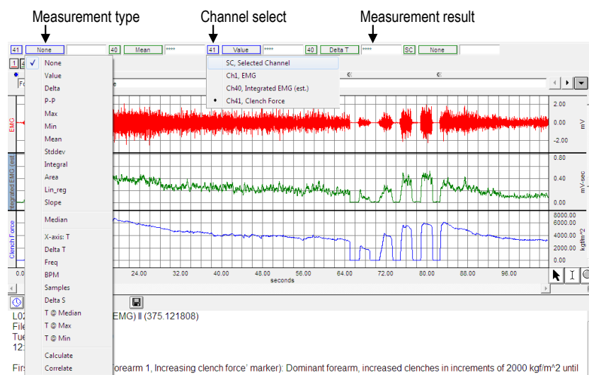
Figure 3.3. Frequently used measurement tools for data analysis
