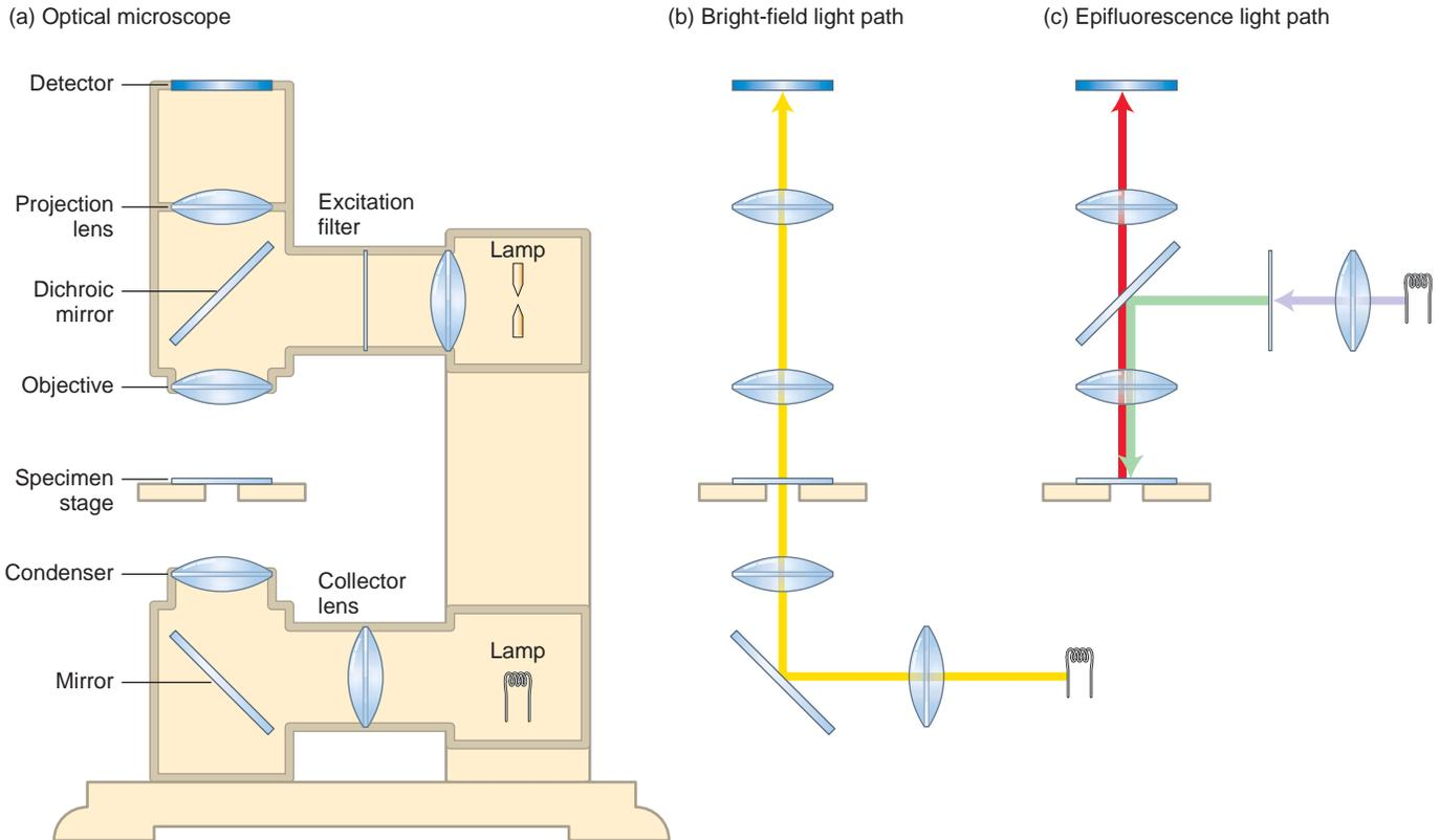
▲ **EXPERIMENTAL FIGURE 5-42** Optical microscopes are commonly configured for both bright-field (transmitted) and epifluorescence microscopy. (a) In a typical light microscope, the specimen is usually mounted on a transparent glass slide and positioned on the movable specimen stage. The two imaging methods require separate illumination systems but use the same light gathering and detection systems. (b) In bright-field light microscopy, light from a tungsten lamp is focused on the
