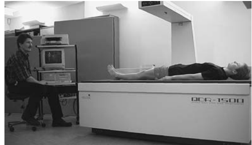
Figure 1.4 Dual energy x-ray absorptiometer procedure for assessing body density and body composition.
