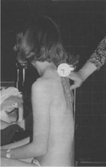
Figure 4.7 A goniometer used to measure the proclive angle, the angle between the spine and vertical at the level of the 7th cervical vertebra.
