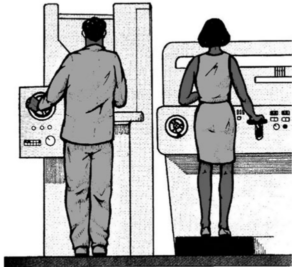
Fig. 11.24 Providing a platform to stand on is helpful to a short operator of a machine designed for a tall user – but note the danger of stumbling (adapted from ILO International Labour Office, 1986)
