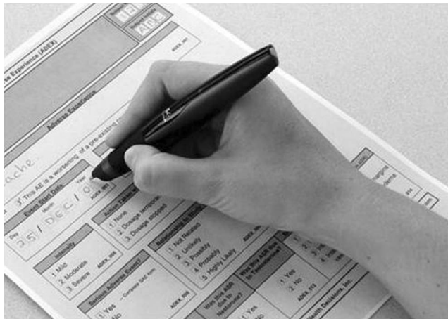
FIGURE 3 A digital pen used for data capture. This method electronically reads in data, eliminating the requirement for manual data entry. (Figure copyright 2006, Health Decisions, Inc. Used by permission.)
