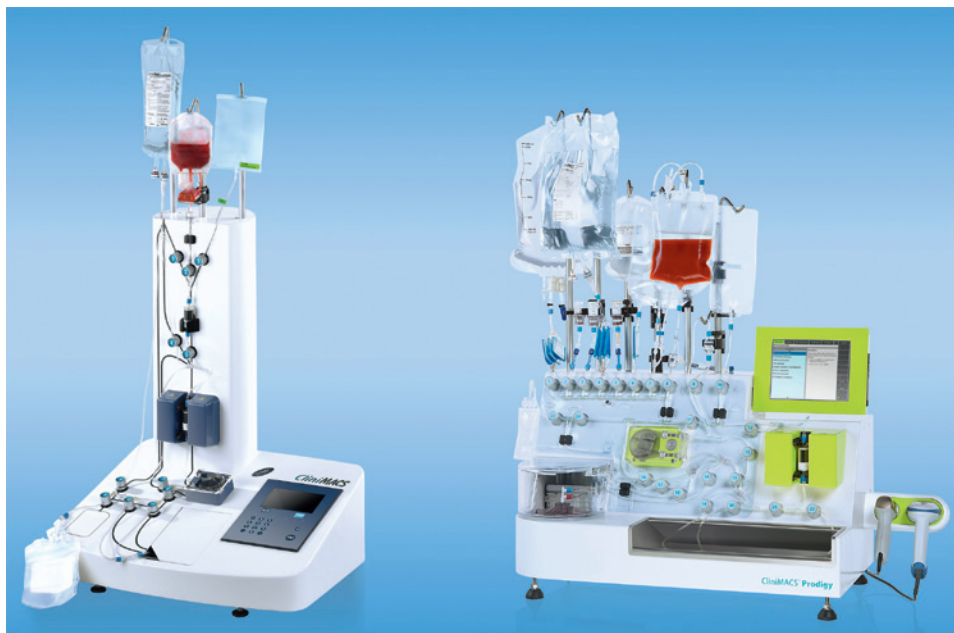
Fig. 97.2 MILTENYI CLINIMACS CELL SEPARATOR AND PRODIGY CELL PROCESSOR. The Prodigy (right side) is a self-contained cell separation and processing device. CliniMACS is a cell separation system using magnetic nanoparticles conjugated with monoclonal antibody to the target antigen. Investigators should determine the status of regulatory approval of these devices before clinical use. (Copyright 2015 Miltenyi Biotec GmbH. All rights reserved.)
