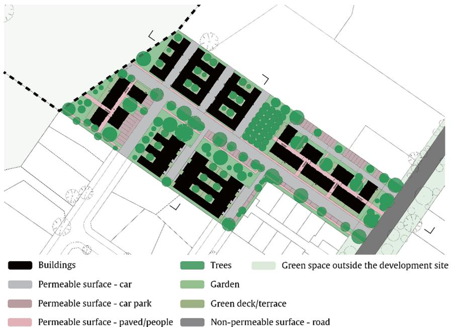
**Fig. 3.3** An example of water-sensitive design for the Salisbury case study. (Source: adapted from Renouf et al. (2020b) and London et al. (2020b), <https://watersensitivecities.org.au/content/project-irp4/>)
