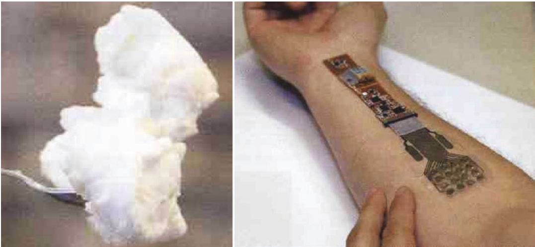
Fig. 14.7 Left: nanocellulose. Right: prototype nanocellulose wound care monitor. (Courtesy of VTT)
