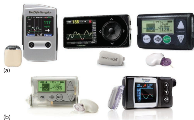
Figure 43.1 Various types of real-time continuous glucose monitors. (a) Stand-alone devices. From left to right: Abbott Freestyle Navigator®, Dexcom Gen4®, and Medtronic Guardian®. (b) Continuous glucose monitors integrated with insulin pumps. Left: Medtronic MiniMed Paradigm Revel and Right: Animas Vibe.
